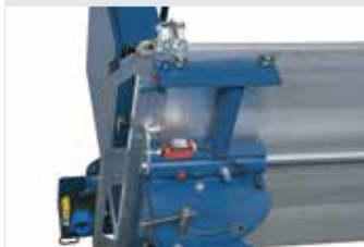
Automatic saw shut-off
